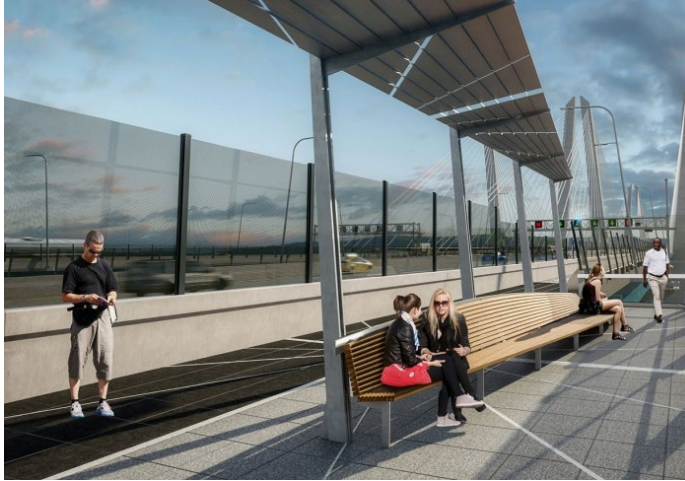
Acrylic Transparent Noise Reduction Panels Mounted on a Traffic Barrier (Tappan Zee Bridge)
