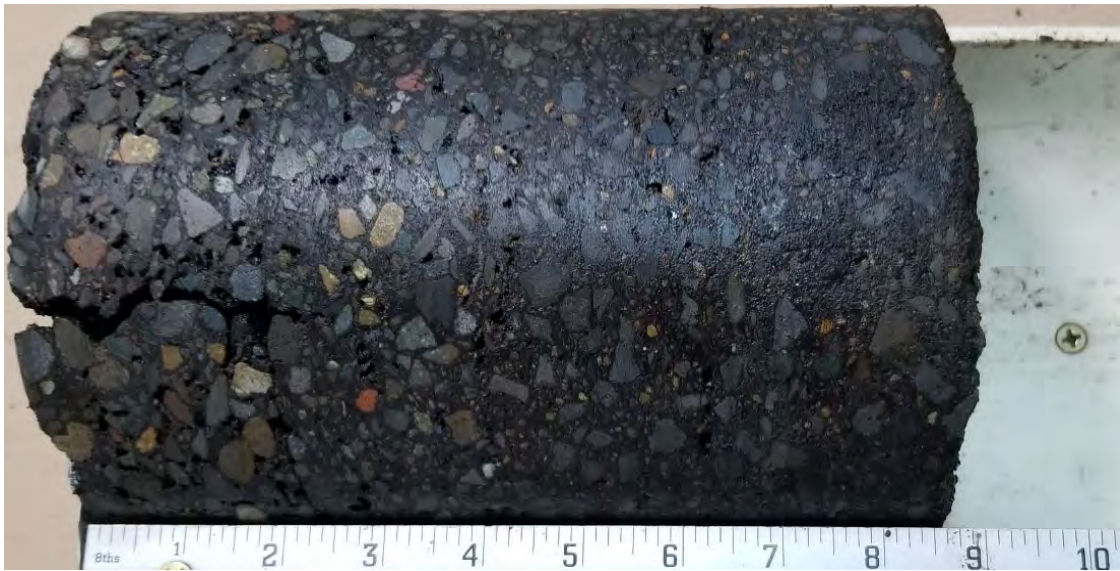
B-1 (Pavement Core Sample, 8.75 in.)
