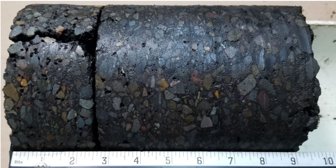
B-3 (Pavement Core Sample, 9.0 in.)
