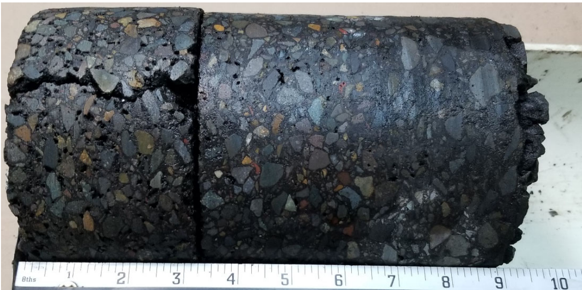
B-2 (Pavement Core Sample, 9.0 in.)
